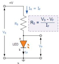
1). series resistor required at 10mA.
