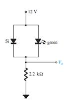
8. Calculate the currents IR1 & IR2 in the configuration shown. Both LEDs have a reverse breakdown voltage of 3 V and an average turn-on voltage of 5 V.
