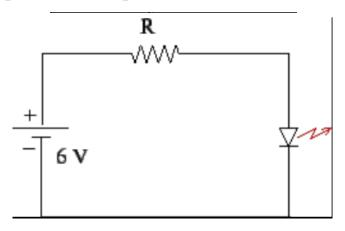
If r is the internal resistance of the LED he current through the resistors is V/(R+r)=0.015 which gives  $R+r=6/0.015=400~\Omega$ . As the drop across LED is 1.6 V, the internal resistance r is  $1.5/0.015=100~\Omega$ . The external resistance to be connected is  $R=400-100=300~\Omega$ . The power rating of the resistor should at least be  $RI^2=300\times 2.25\times 10^{-4}=77.5$  mW.
